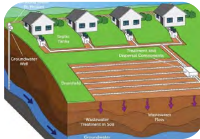
Large On-site Sewage Systems (LOSS)
