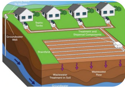
Large On-site Sewage Systems (LOSS)
