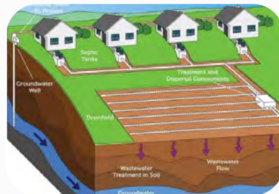
Large On-site Sewage Systems (LOSS)
