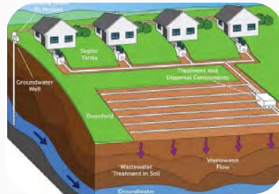
Large On-site Sewage Systems (LOSS)
